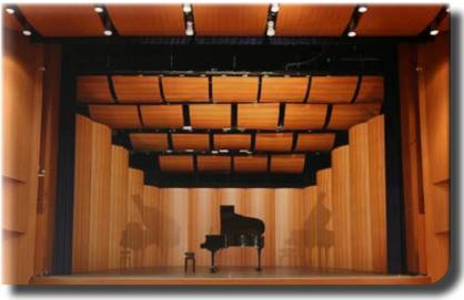
Proper use of acoustical materials helps to define the sound quality of the room. Our Symphony panels curved shape disburses the sound evenly across the audience, our panel materials are completely customizable to fit into any aesthetic design.
